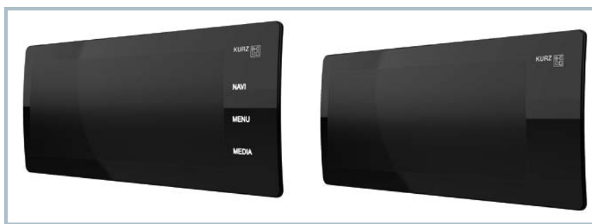
Fig. 2. Function and decor rolled into one: at Fakuma, a complete ten-inch HMI display in dead front design, with integrated electronics and top coat for scratch resistance, takes shape on the PX 320 in one production step (© Leonhard Kurz)
