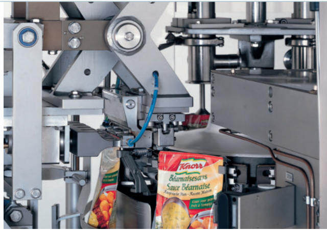
Fig. 7. Ultrasonic sealing module for top sealing of standup pouches
