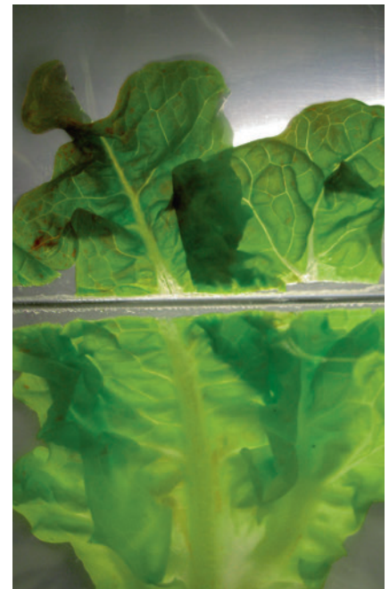
Fig. 6. An extreme example of reliable sealing of surfaces contaminated by the product
