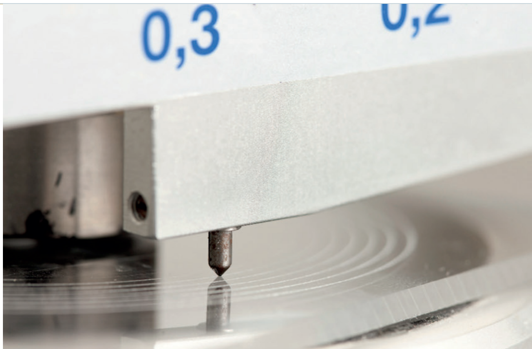
The surface exhibits high scratch hardness in the Erichsen test
