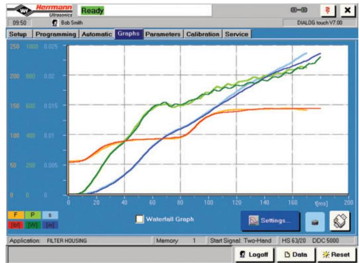
Fig. 8. Screenshot showing joining velocity
