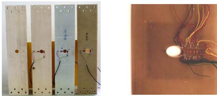
Figure 7: Strain gauge positioning on the timber-GFRP structures and GFRP specimens
