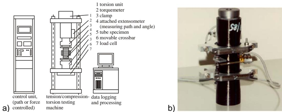
Figure 4: Tension/compression-torsion failure tests
