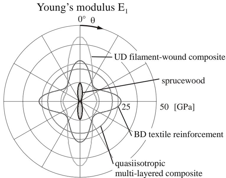
Figure 3: Comparison of direction-dependent elasticity modules ( $\theta = 0^\circ$ : fibre direction)
