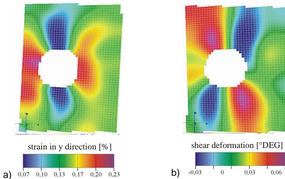
Figure 8: Strain fields of UD-GFRP timber structures subject to tension
