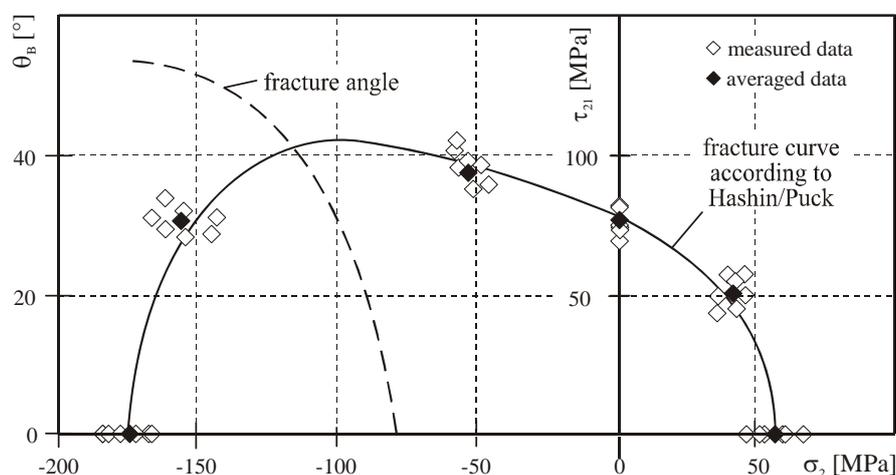
Figure 5: Strengths, failure curve and fracture angle for tangentially wound GFRP tube specimens
