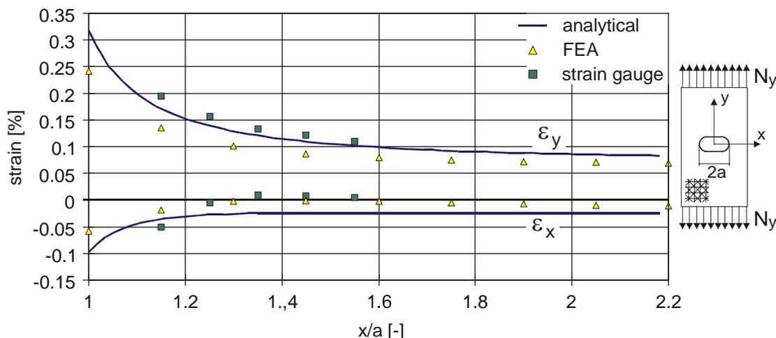
Figure 9: Comparison of calculated and measured strain for a quasi-isotropic composite
