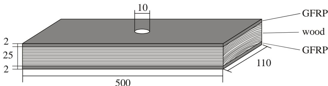
Figure 1: Schematic representation of a hybrid GFRP/ wood sample with circular hole
