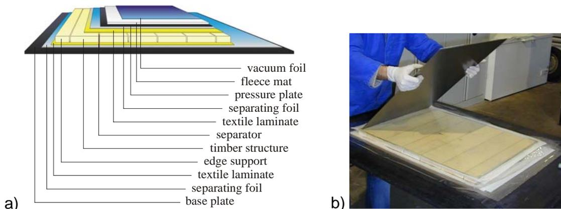
**Figure 6:** *Manufacture of textile-reinforced timber structures by means of vacuum autoclaving method*
