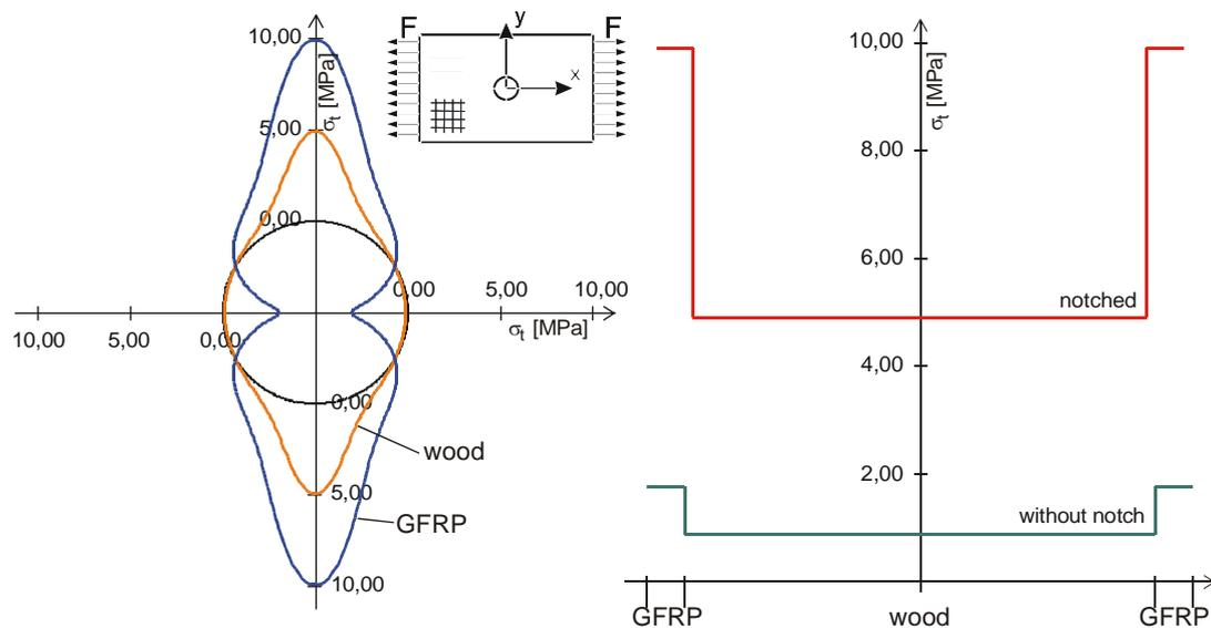
Figure 2: Analytically-calculated tangential stress for sprucewood with glass fibre-reinforced plastic (GFRP) textile reinforcement
