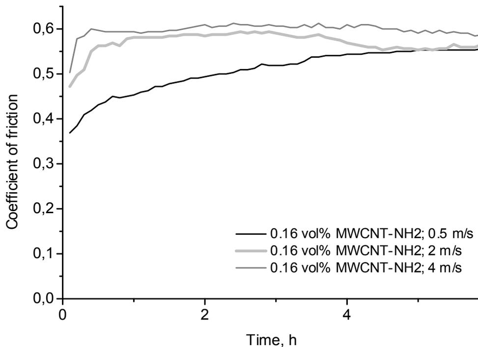
Figure 4: The coefficient of friction of epoxy nanocomposites during sliding at 1MPa
