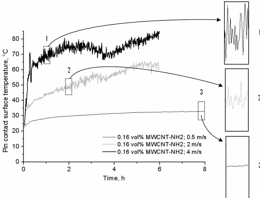
Figure 2: Contact surface temperature versus time of epoxy nanocomposites during sliding at 1MPa
