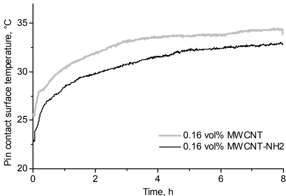
Figure 5: Contact surface temperature of surface modified and non-modified CNT nanocomposites during sliding at 1 MPa pressure, 0.5 m/s speed
