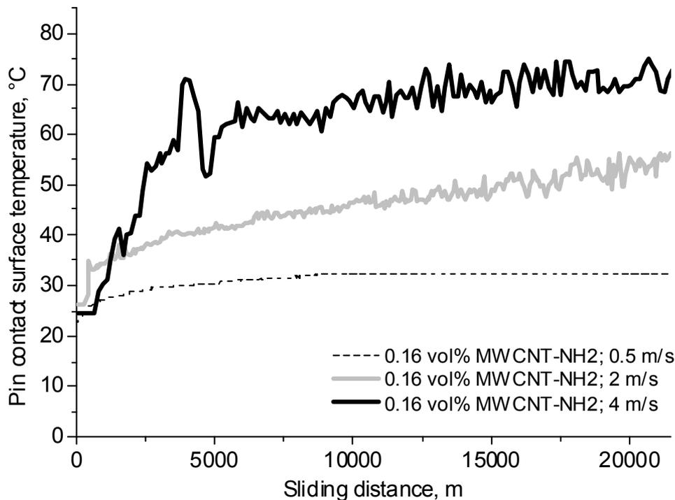
Figure 3: Contact surface temperature of epoxy nanocomposites during sliding at 1MPa as a function of sliding distance
