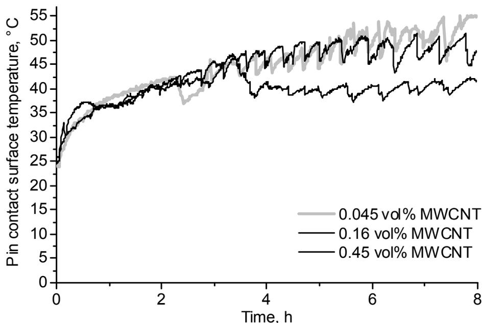
Figure 7: Contact surface temperature of CNT-epoxy nanocomposites during sliding at 1 MPa pressure, 1 m/s speed
