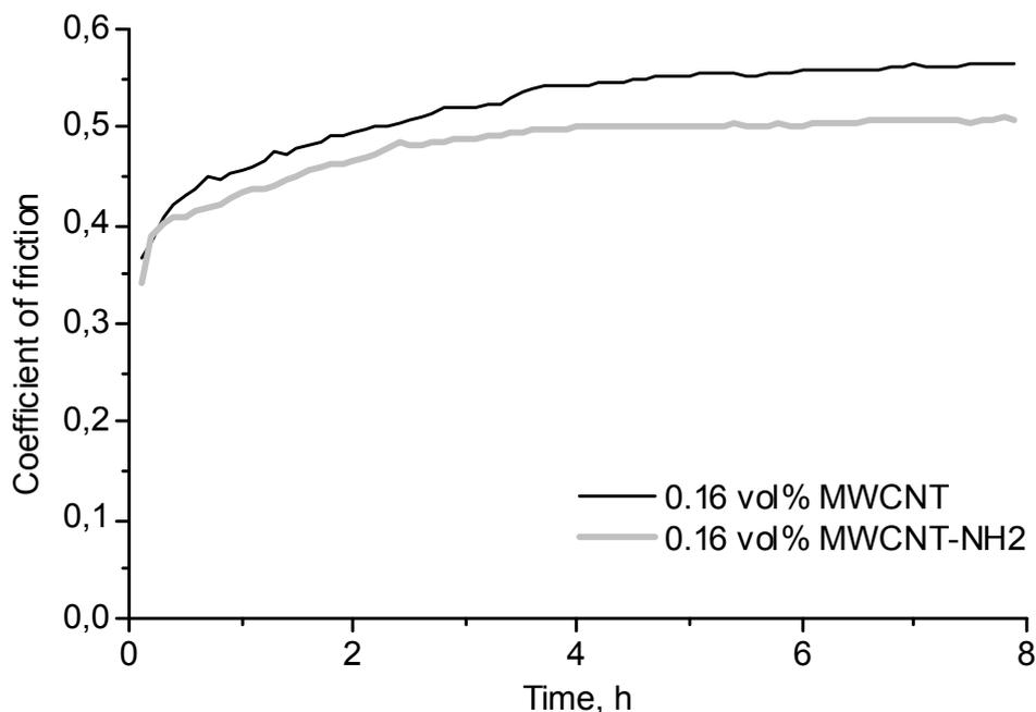
Figure 6: The coefficient of friction for modified and non-modified CNT nanocomposites during sliding at 1 MPa pressure, 0.5 m/s speed
