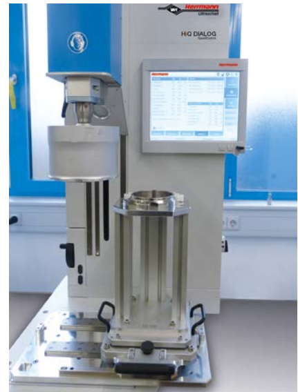
Fig. 4. HiQ Dialog 6200: The ultrasonic welding machine has a vertically adjustable tool holder and can display the weld course graphically on its 15-inch screen (© Herrmann Ultraschall)
